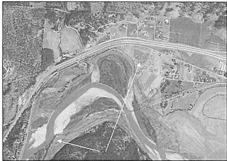
Figure 14. Areas in Reach 4 where CMZ extends beyond 100-year floodplain (yellow arrows).
